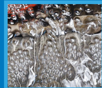
9. Documented leakage / leak test
